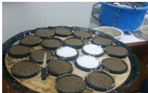
Figure 2. Preparing soil and placing samples on Bar extractor and Porous plate extractor
